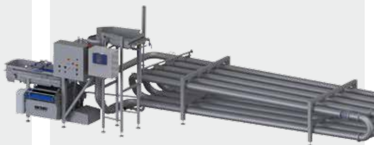
VORTEX-line for germ reduction + prolongation of shelf life of fresh-cut products
